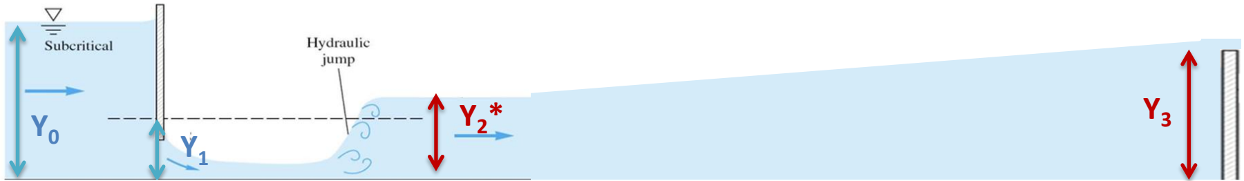
Figure 11 : Schéma d'un ressaut hydraulique, d'après Mikolaj Szydlarski, Chiara Simeoni. Numerical simulation of shallow water equations and comparison with experimental data
